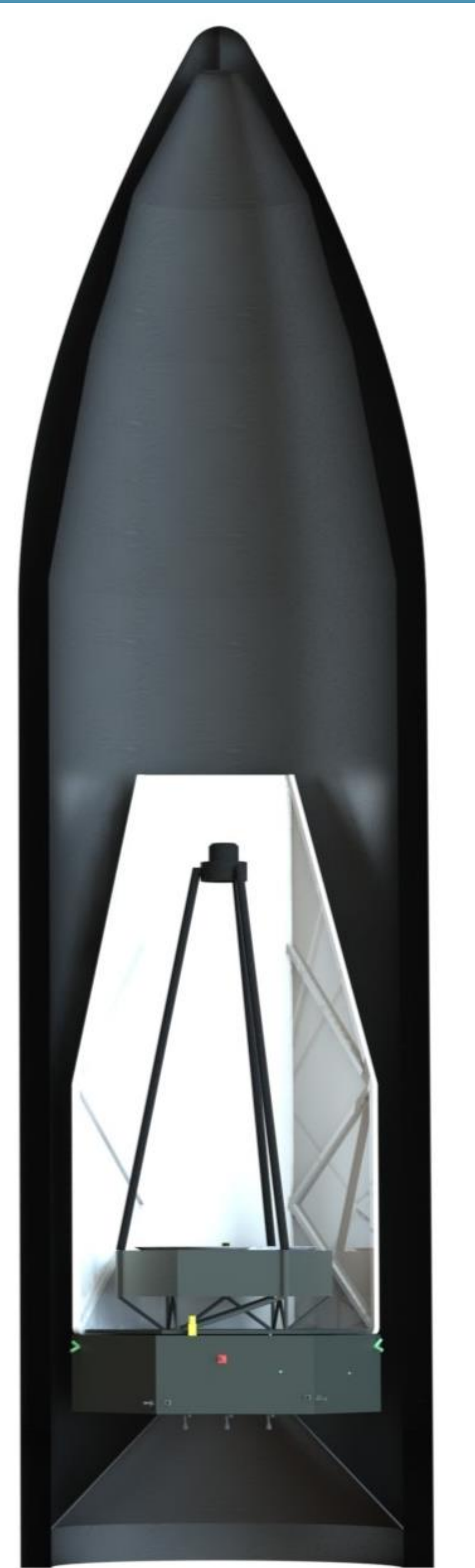
Figure 7: Exodux spacecraft placed in Ariane 62 fairing.
